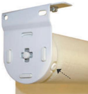
Ⓐ If you have lost tension on the shade, push the locking spring pin back in. This will ensure the shade spring will not unwind completely when removing the shade from the brackets for adjustment.
