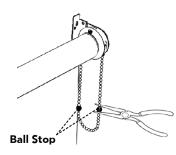
• On the opposite side, place a ball stop on the bead closest to the clutch. Use needle nose pliers to clamp ball stop in place.
