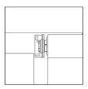
B). Depress the coupling plunger and then locate and secure fixed end into adjacent shade.
