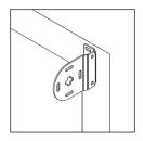
B). Place a coupler bracket at the intermediate point approximately 1/16" less than the size taken, ensuring the central face of the intermediate bracket lines up accordingly.
